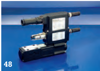
① servocylinder with position transducer, ② servoproportional valve DLHZO with ③ integral digital controller Z-RI-TEZ, ④ position feedback signal, ⑤ connections to electric power, electronic signals and fieldbus
